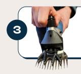
Turn on the clippers to prepare for clipping, gradually tighten the blades until they start clipping
